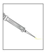
Prior to dispensing into the anchor hole, squeeze out a 10cm length bead of material and discard. The adhesive should now have a consistent, uniform color indicating correct mixing is occurring.
