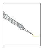
Prior to dispensing into the anchor hole, squeeze out a 10cm length bead of material and discard. The adhesive should now have a consistent, uniform color indicating correct mixing is occurring.
