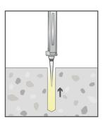
With the cartridge nozzle tip at the base of the cleaned drill hole, inject adhesive until the hole is approximately 2/3 full. Slowly withdraw the nozzle from the hole whilst injecting, keeping the nozzle tip immersed in the adhesive. This will avoid creating air pockets within the adhesive.
