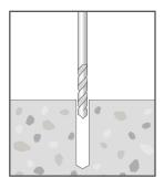
Drill hole into substrate to the specified diameter and depth using a rotary hammer drill and correctly sized carbide bit.
