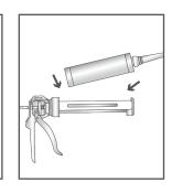
Insert the cartridge into the dispenser and screw the correct mixing nozzle onto the cartridge.
