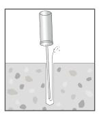
Blow out from the base of the drill hole at least 2 times until removed air is free of noticeable debris. For drill holes up to 18mm diameter - a manual blower pump may be used to clean the hole. For larger diameter holes - compressed air cleaning must be used and may also be used for smaller holes.
