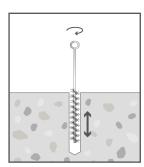
Brush 2 times with a wire brush (its diameter should be greater than the drill hole diameter) - inserting the brush to the base of the hole and withdrawing it with a twisting motion.
