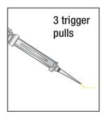
Prior to dispensing into the anchor hole, squeeze out 3 trigger pulls of material and discard. The adhesive should now have a consistent, uniform color indicating correct mixing is occurring.
