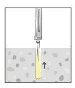
With the cartridge nozzle tip at the base of the cleaned drill hole, inject adhesive until the hole is approximately 2/3 full. Slowly withdraw the nozzle from the hole whilst injecting, keeping the nozzle tip immersed in the adhesive. This will avoid creating air pockets within the adhesive.
