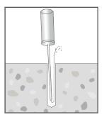
Blow out from the base of the drill hole at least 2 times until removed air is free of noticeable debris. For drill holes up to 18mm diameter - a manual blower pump may be used to clean the hole. For larger diameter holes - compressed air cleaning must be used and may also be used for smaller holes.
