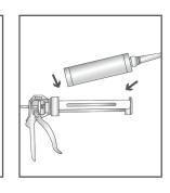
Insert the cartridge into the dispenser and screw the correct mixing nozzle onto the cartridge.
