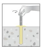
Ensure the anchor stud is clean and free of contaminants, grease etc. Push the anchor stud into the adhesive - slowly rotating the stud until it is seated against the base of the hole. An excess of adhesive around the top of the hole indicates sufficient material was injected into the hole, otherwise remove the anchor stud and renew the hole with adhesive.
