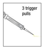
Prior to dispensing into the anchor hole, squeeze out 3 trigger pulls of material and discard. The adhesive should now have a consistent, uniform color indicating correct mixing is occurring.
