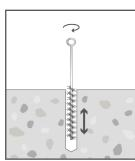
Brush 2 times with a wire brush (its diameter should be greater than the drill hole diameter) - inserting the brush to the base of the hole and withdrawing it with a twisting motion. If no resistance is felt during this step, the brush is worn replace it.
