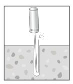
Blow out from the base of the drill hole at least 4 times until removed air is free of noticeable debris. For drill holes up to 22mm diameter - a manual blower pump may be used to clean the hole. For larger diameter holes - compressed air cleaning must be used and may also be used for smaller holes.
