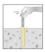
Ensure the anchor stud is clean and free of contaminants, grease etc. Push the anchor stud into the adhesive - slowly rotating the stud until it is seated against the base of the hole. An excess of adhesive around the top of the hole indicates sufficient material was injected into the hole, otherwise remove the anchor stud and renew the hole with adhesive.
