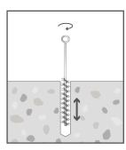
Brush 4 times with a wire brush (its diameter should be greater than the drill hole diameter) - inserting the brush to the base of the hole and withdrawing it with a twisting motion. If no resistance is felt during this step, the brush is worn - replace it.
