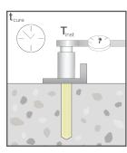
All steps prior must be completed within the working time of the adhesive. Protect the anchor from disturbance until the full curing time has been reached. Once full cure is achieved, carefully place the fixture and apply the specified installation torque.
