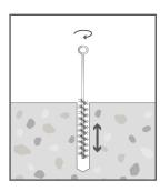
Brush 4 times with a wire brush (its diameter should be greater than the drill hole diameter) - inserting the brush to the base of the hole and withdrawing it with a twisting motion. If no resistance is felt during this step, the brush is worn - replace it.
