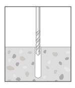
Drill hole into substrate to the specified diameter and depth.
