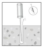
Clean the hole using the following sequence with a blower pump and correctly sized wire / nylon brush:
