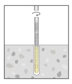
Using a power tool and the driver bit supplied with the studs, rotate & drive the anchor stud into the capsule until the anchor stud bottoms out in the hole. Stop driving and remove tool / driver at this point. PROTECT THE ANCHOR FROM DISTURBANCE UNTIL THE CURE TIME HAS ELAPSED.
