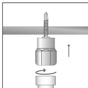
Attach the correct sized socket driver to the hanger and drive until the anchor is securely fastened, take care not to overdrive.
