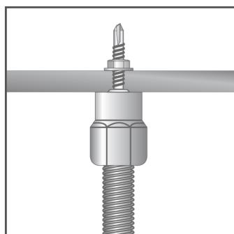
Secure the hanger by fitting the supplied nut.
