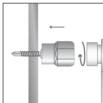
For additional connection strength thread nut supplied onto the hanger from behind the metal substrate.
