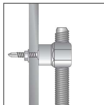
Ensure the threaded rod is fully threaded through the fastener. Secure rod with M10 nut(s) for additional security.
